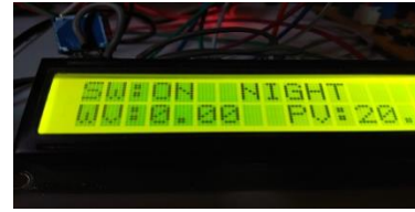
Fig. 7. Display of mode of switch and intensity of light in room
