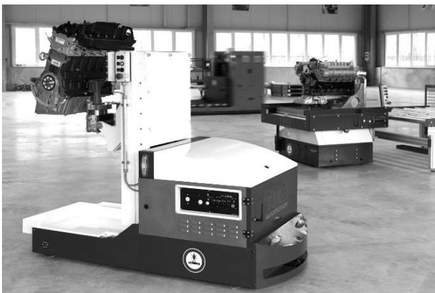
Fig. 1: Automated Guided Vehicle (TMS Automotion GmbH, Austria)
