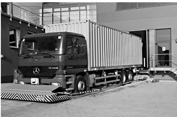
Fig. 3: Automated motor truck (Götting KG, Germany)
