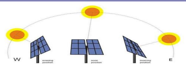
Types of solar tracking system : 1. Single axis solar tracking system
