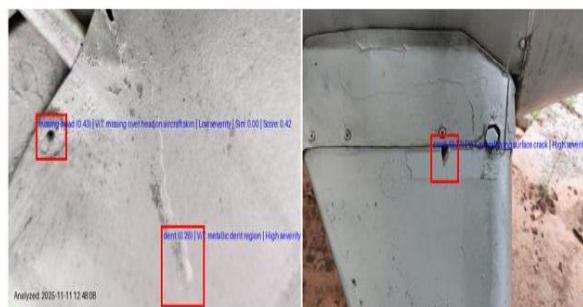
Fig. 6. Severity-Level Visualization for Aircraft Defects
