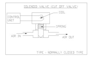
In our Work separate solenoid valve is used for flow direction of vice cylinder. It is used to flow the air from compressor to the single acting cylinder.
