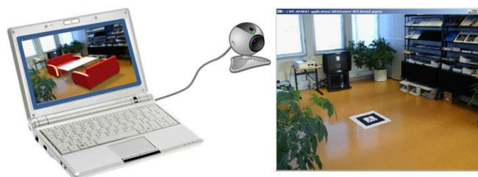
Figure 1. Example of a simple augmented reality system setup.
