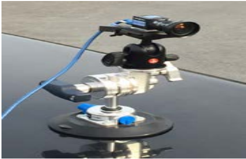
Figure 2: Rear car with a single camera fixed on the rooftop
