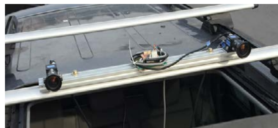
Figure 1: Picture of the front car equipped with a stereo vision system
