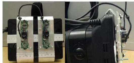
Figure 5: Camera mounted on Oculus Rift
