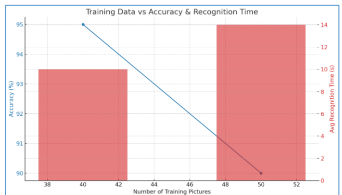
Fig.3. Training Data vs Recognition Time. The blue line represents accuracy (%), showing a decrease as the number of training pictures increases. The red bars represent average recognition time (s), which increases with more training pictures.
