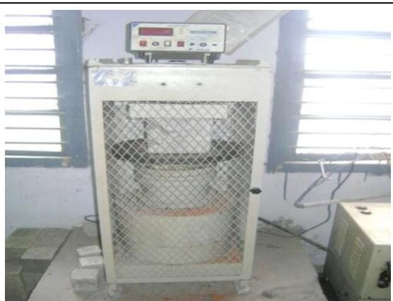
Figure 3.1: Compression Testing Machine (CTM)
