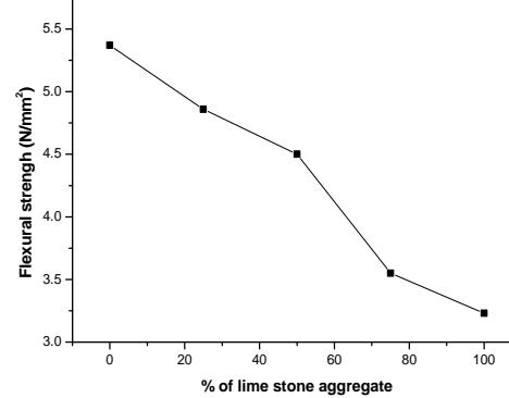
Figure 4.4: Flexural strength vs. % of lime stone aggregate.
