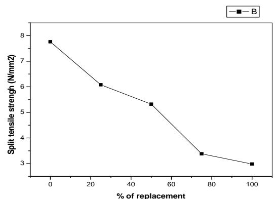
Figure 4.3: Split Tensile Strength vs % Lime stone aggregate
