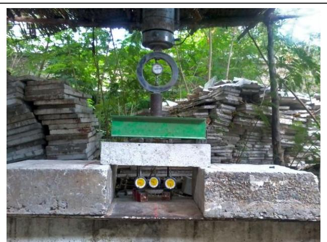
Figure 3.3: Flexural Strength test setup
