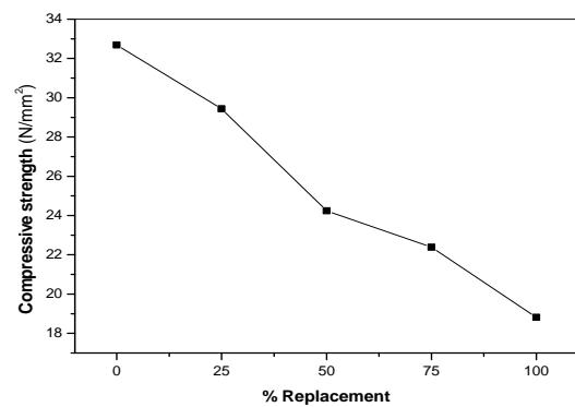
Figure 5.2: Compressive Strength vs. % Lime stone aggregate
