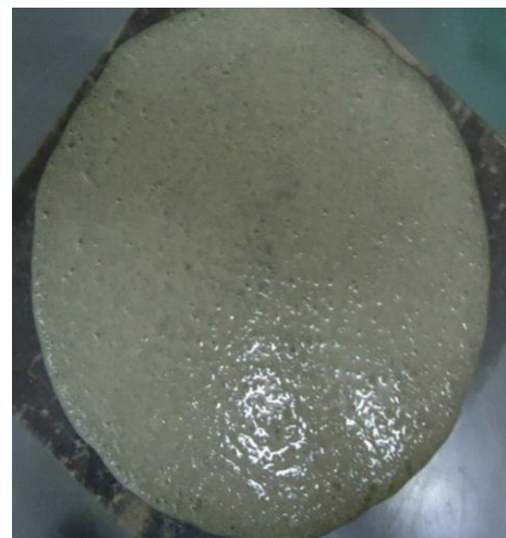
Fig 3. Slump of self-compacting concrete
