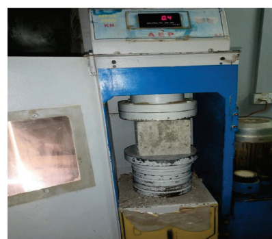
Fig - 6: Compressive Strength machine
