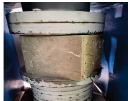
Fig - 13: Crack Pattern at 0.05% Polypropylene Fiber Content
