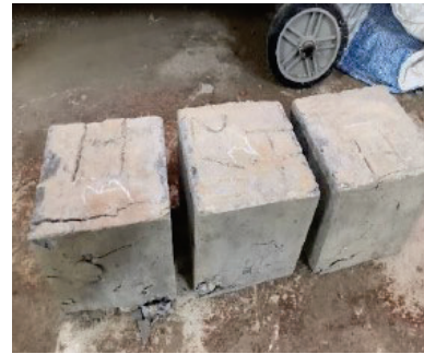
Fig - 12: Crack Pattern at 0.0% Polypropylene Fiber Content
