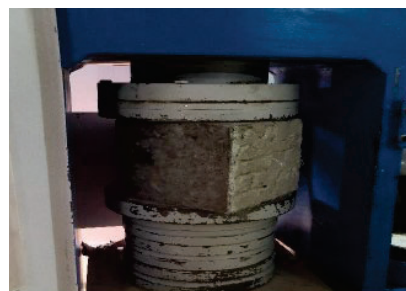
Fig - 15: Crack Pattern at 0.25% Polypropylene Fiber Content
