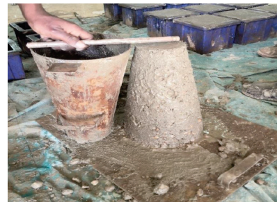
Fig - 4: Slump test
