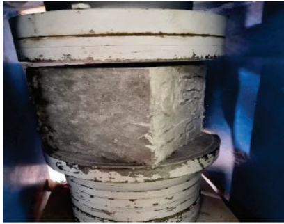
Fig - 16: Crack Pattern at 0.35% Polypropylene Fiber Content
