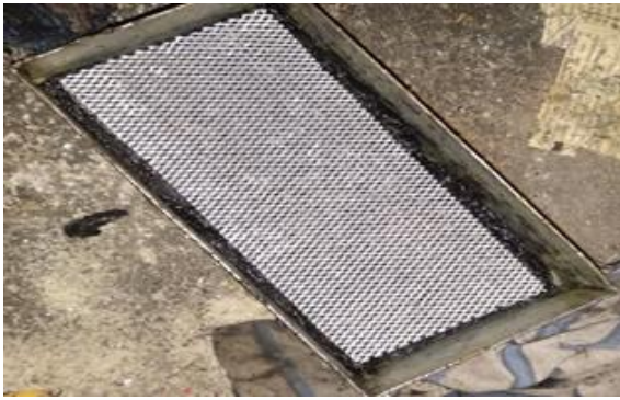
Fig. 6: Aluminium mesh of size 18.5x8.5cm
