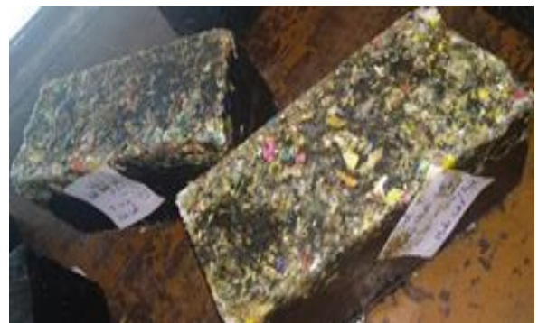
Fig. 10: Test 7 brick with max compressive load capacity and plastic coated over the surface
