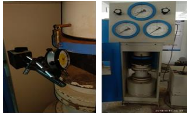
Fig. 8.1.a, Fig. 8.1.b: Compressive load testing machine and dial gauge used for testing the bricks
