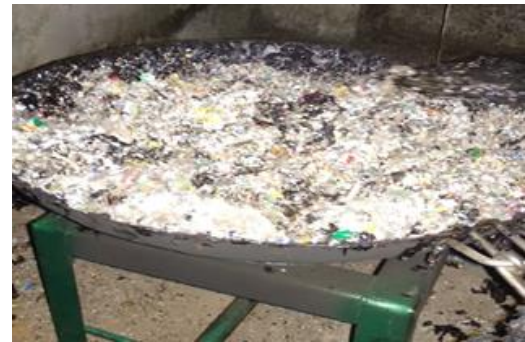
Fig. 5: Shredded plastic of size 4-10mm
