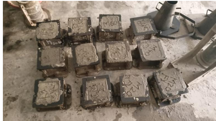
Figure 6.1 Concrete Cube Casting
