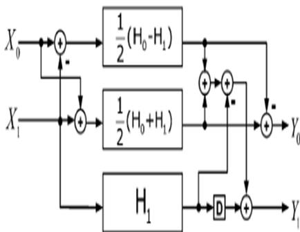
Fig.3 Proposed Two- Parallel FIR filter implementation using the FFA
