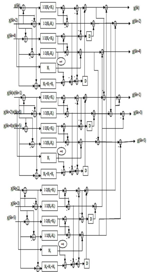
Fig.5 Proposed Six- Parallel FIR filters implementation using the FFA.
