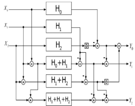
Fig.2. Three-parallel FIR filter implementation using the FFA.
