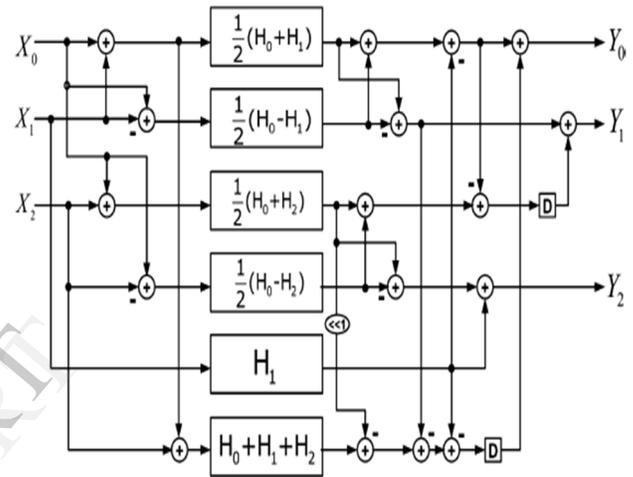
Fig.4 Proposed Three- Parallel FIR filter implementation using the FFA
