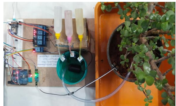
Fig 7. fertilization and irrigation system
