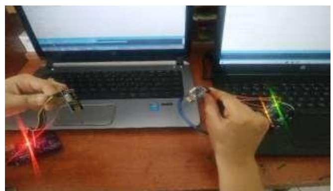
Fig.5:- Practical image of RF compact module using nRF24L01
