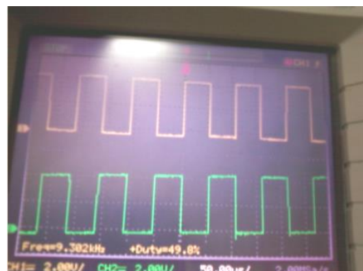
Fig. 5 Generation of PWM pulses by Arduino
