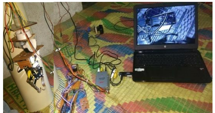
Figure8. Gripper mechanism and visual feedback from the camera
