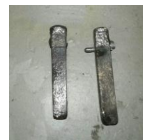
Fig 2.4 Samples after partial re-melting and holding for a specified time.
