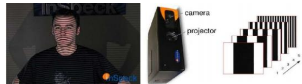
Figure 3: Light based 3d body scanning.
