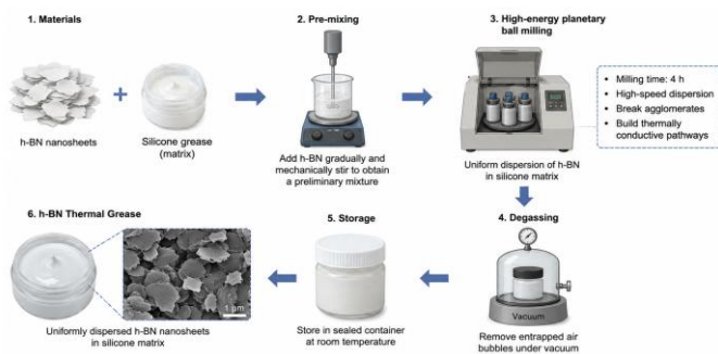
Fig. 1. Preparation of h-BN Thermal Grease
