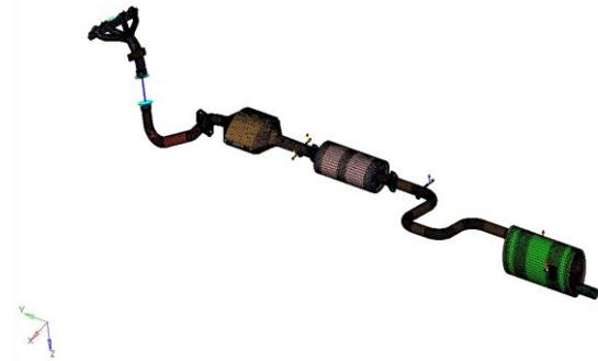
Fig 4.3: Finite Element Model of the exhaust system
