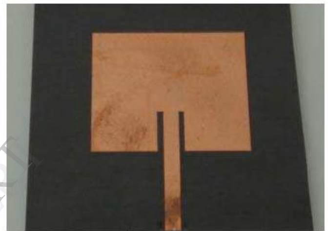
Fig 5 fabricates microstrip patch antenna
