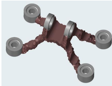
Fig.7. Geometry of the Model after weight optimized Inspire-Optistruct software was used to optimize the design and make the bracket suitable for Additive manufacturing technology.
