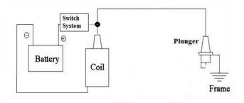
The Anti-accident Ignition System connected is to Battery, Ignition Coil, Plunger. The switch system is connected to the battery at one end to the other end it is connected to ignition coil as well as to the plunger with the help of node. The plunger is earthed with the help of frame.
