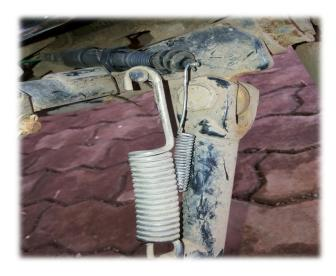
The main function in the mechanism which has been implemented in the two wheeler is that when the stand is at ON position the circuit get break and the current from the battery doesn't flow through ignition coil rather than current passes through the earthling which is provided by the plunger with the help of chassis. This will pass the voltage current to the rubber parts of the vehicle where the current gets absorbed as well as by the help of side stand current will flow into the earth surface.
