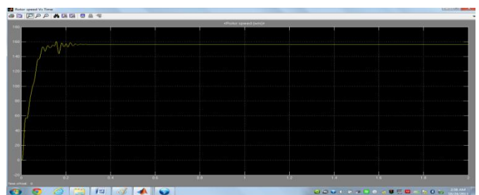
Figure 11.4: rotor speed Vs Time Graph for Medium rotor Resistance
