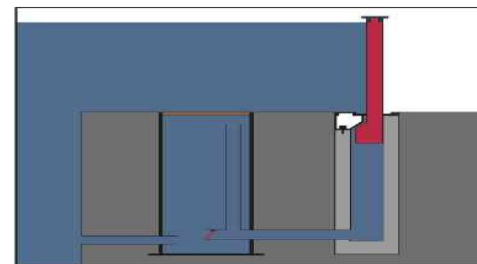
Fig.5 Hydrostatic ensures the barriers stay in until flood subsides.
