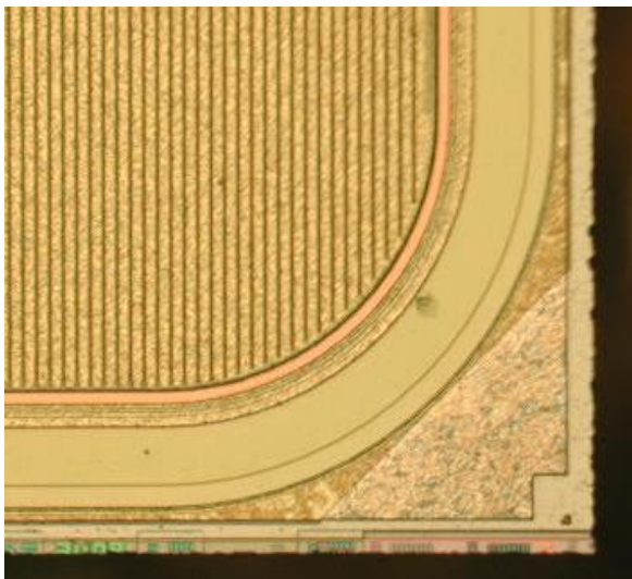
Fig. 7. IGBT isolation region without RB capability.
