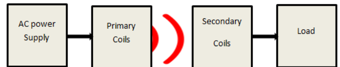
Fig.1. Block Diagram of Magnetic Induction
