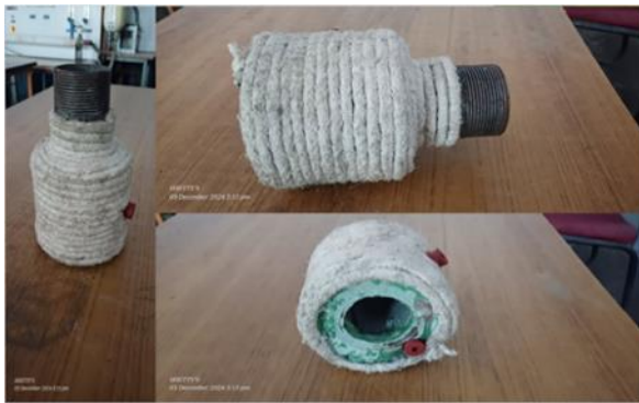
Figure 2.1. heat storage device connected to the Engine exhaust
