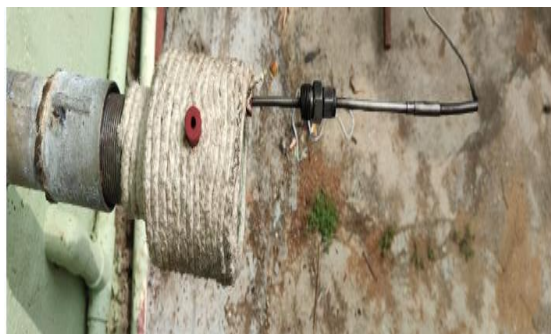
fig 2.3- experimental setup connected to the Engine exhaust with thermocouple
