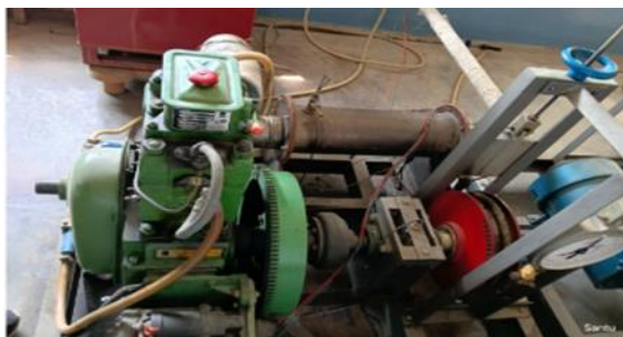
fig 2.3 4-Stroke diesel Engine setup for experimentation
