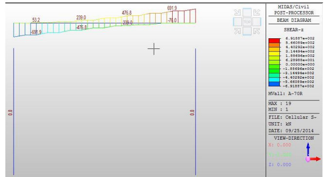
7 M SPAN SHEAR FORCE VOIDED
