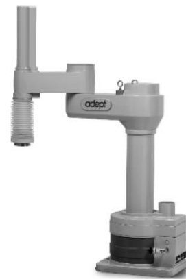
Figure 5: Adept Technology Inc industrial robot, The AdeptOne XL
