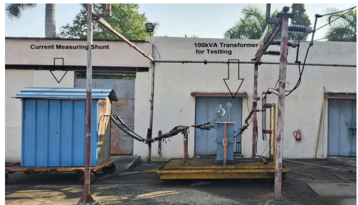
Figure 1. Short circuit Test Setup for Transformer
