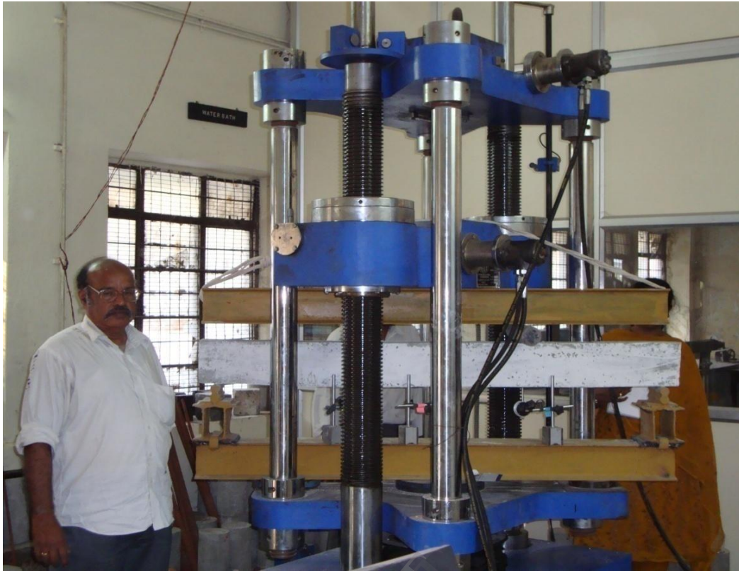
Plate 1 Computerized universal testing machine with set up
