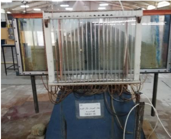
Fig. 2. Alignment of seepage and permeability model
