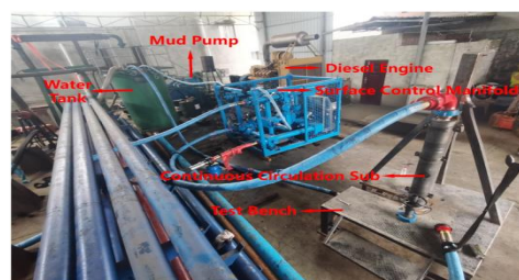
Figure 10. Pressure Loss Test Experiment for the Valve-Based Continuous Circulation Drilling System
