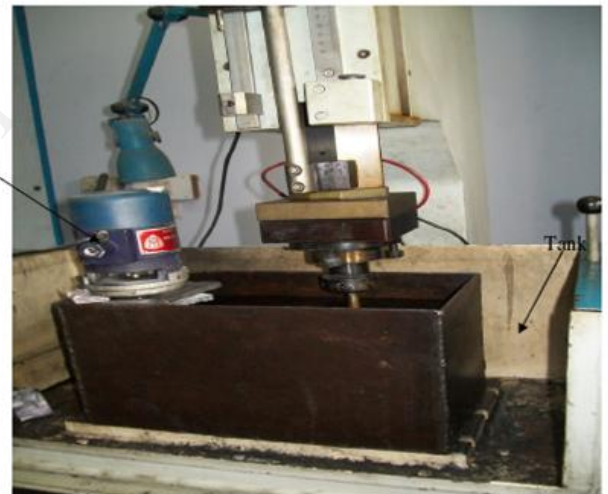
Fig. 2: Dielectric tank with Stirrer attachment
