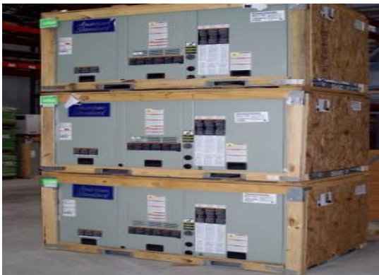
Fig no.2.3 A stack of roof top units for mid-sized commercial buildings.
