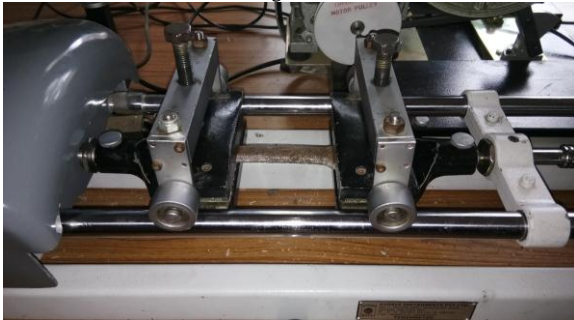
Fig 2.2 Sample Loaded Condition For Tensile Testing
