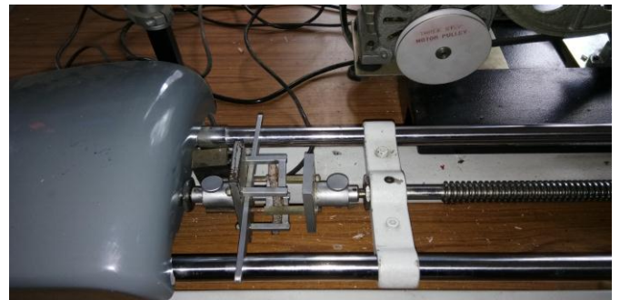
FIG 2.5 Sample loaded condition for flexural testing
