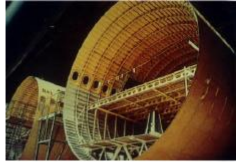
Fig. 1.12- Aircraft internal structure includes extrusions and plate of 2xxx alloys.
