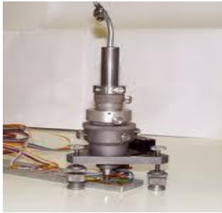
Fig 1.9: Hole Drilling Machine
