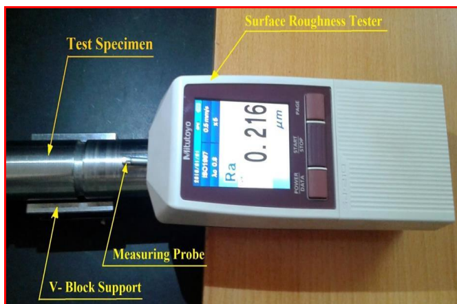
Figure 9: Photograph of Surface Roughness testing set up
