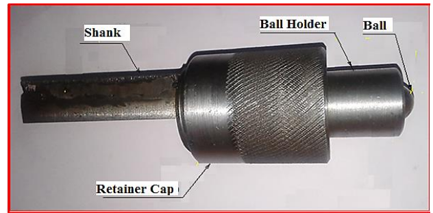
Figure 4: The ball burnishing tool
