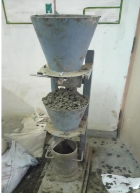
Fig.4 Compaction factor test apparatus
