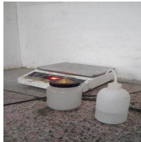
Fig.3 Specific gravity test by pycnometer
