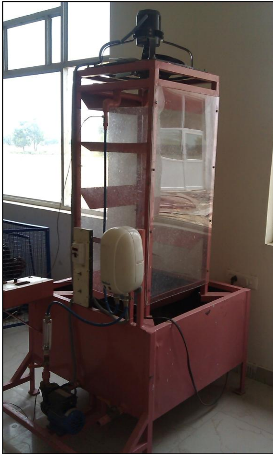
Figure 2.1 Water Cooling Tower
