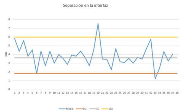
Fig. 9. Separation plot on the interface
