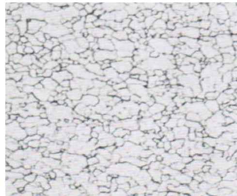
Fig.7. Microstructure after annealing mode 1, reduction 50%
