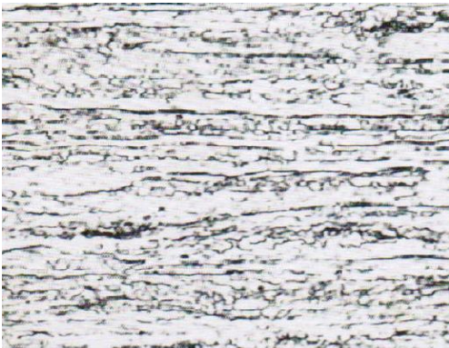
Fig.9. Microstructure after annealing mode 3, reduction 80%
