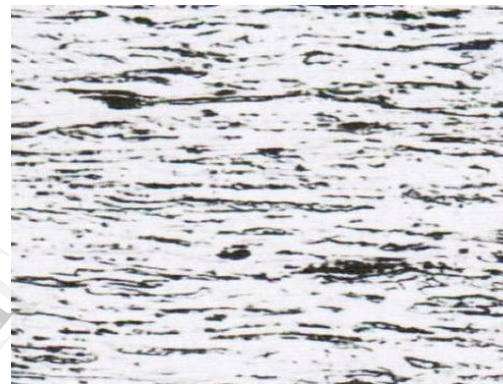
Fig.6. Microstructure after 80% reduction
