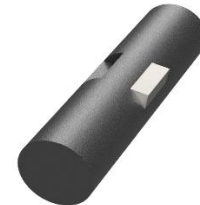
Fig. 3. Kennedy Key fitted in keyway in a shaft
