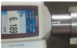
Fig.5 Stylus Movement on Work piece Material
