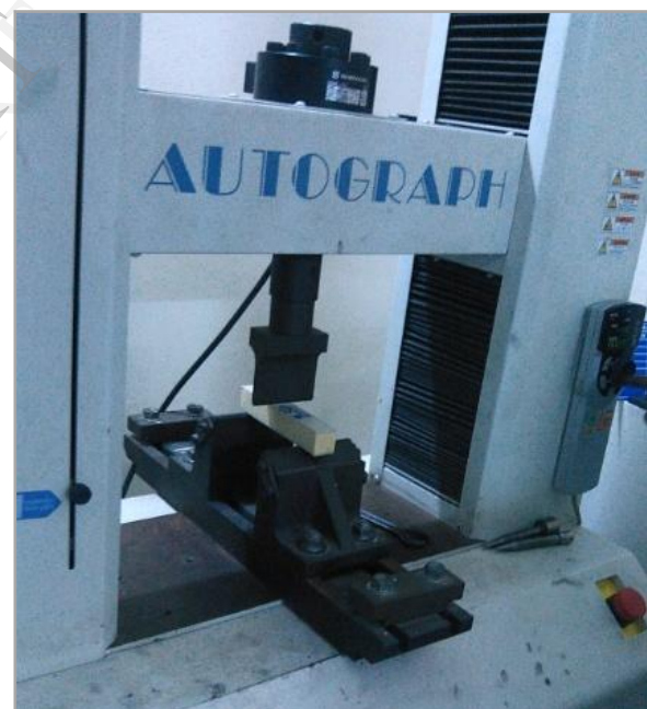
Fig.7. Experimental setup for bending test
