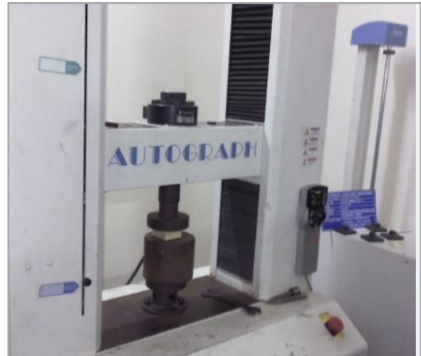
Fig.6. Compressive Tests on UTM
