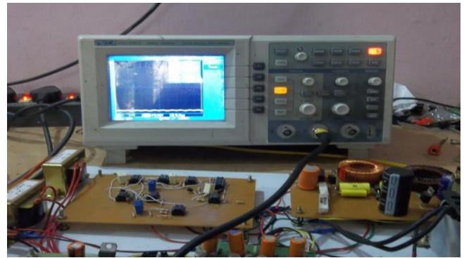
Fig.16 Steady Output voltage of -36V with a change in duty ratio
