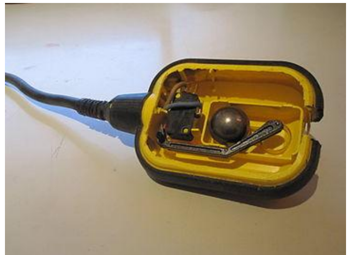
Fig.11. Float switch in ON condition
